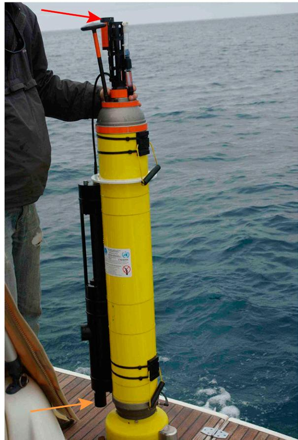
FIG. 1. Photograph of Mediterranean A float after recovery near BOUSSOLE. The optics package is the blackbody attached to the side of the float. The radiometers are marked with arrows (red: downwelling irradiance, orange: upwelling radiance). (Photograph by Florent Besson.)
